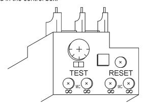
Figure 14. Over Current Relay
